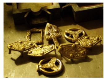
After curing the clay in an oven, I sandcast my belt parts, first making a copy of the clay in pewter, cleaning up the pewter masters, then casting bronze copies from the pewter masters. Here are some of the rough castings, fresh off the sprue. Part of the sand-casting mold frame is visible behind them.
